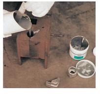
**ALUMINIUM LIQUID** Pourable aluminium filled liquid epoxy for casting, filling duties or in the repair of aluminium castings and equipment. Non rusting and easy to machine, drill or tap. Use to fill voids and holes in aluminium liners and castings, produce high quality fittings and fixtures or to reform damaged aluminium components.
